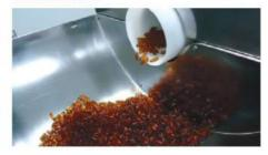
Designed with high efficiency blowers and variable speed for all buckets, the tumble dryers are also suitable for manufacturing different products on the same machine.
