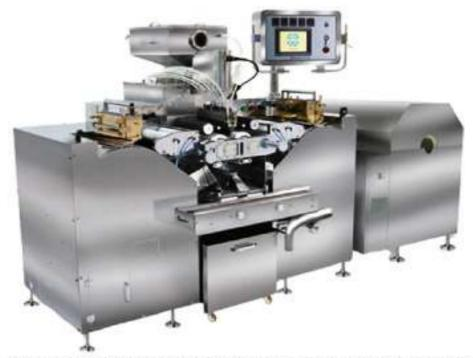
The **BCM-GB6** encapsulation system installed can be used to produce soft gel capsules of various shapes and sizes. Even the products which are oil-based and paste-based can be produced on the same system.
