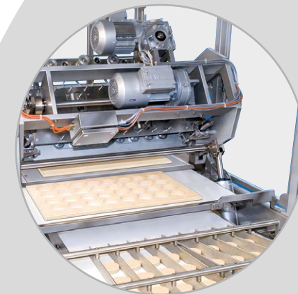
Round Wafer Cutting Machine For the production of cream-filled round wafer sandwiches.
