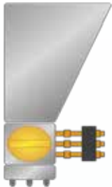
Basic depositor with Mono pump system
